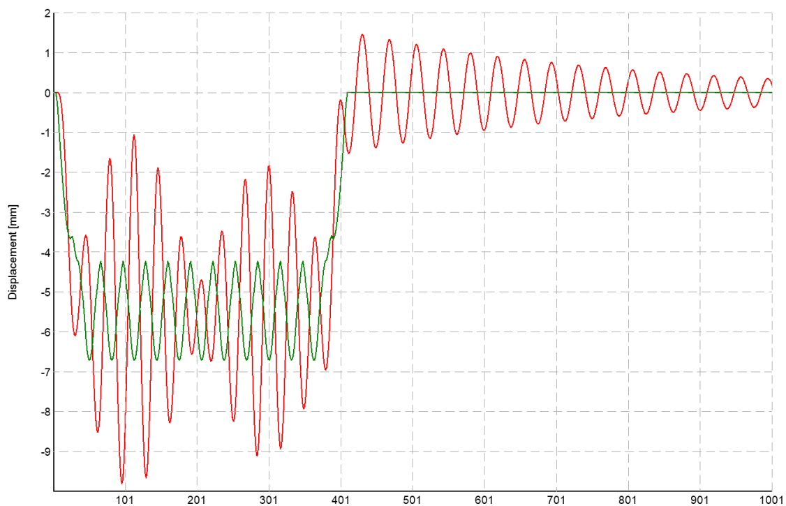
Figure 22 – The dynamic and static displacements of the mid-span in function of force positions with v_2 velocity in FEM-Design in case b)
