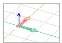
The thin arrows show the axes of the Global (or World) Coordinate System (WCS). The position of the origin and directions are fixed.
