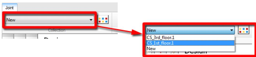
Any joint in *Collection* can be displayed in a separate dialog along with a 3D model of it. In this dialog the user can rename, copy or delete the joints.
