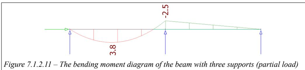
Figure 7.1.2.11 – The bending moment diagram of the beam with three supports (partial load)
