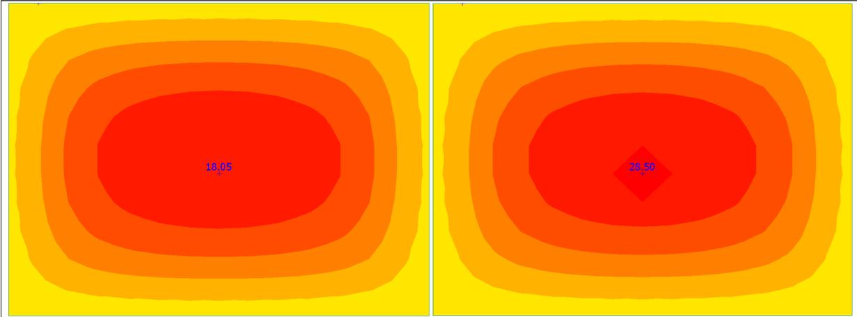
Figure 2.2.3 – The  $m_x$  [kNm/m] moment with 1<sup>st</sup> and 2<sup>nd</sup> order analysis
