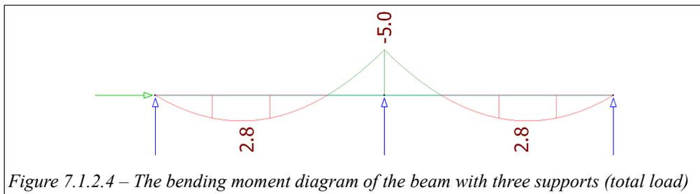
When the middle support only bear tension (second part of this case) basically under the total vertical load (Fig. 7.1.2.1) the middle support is not active (support nonlinearity). Therefore it works as a simply supported beam with two supports. The deflection, the shear forces and the bending moments are the following:
