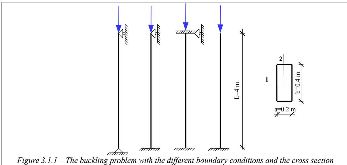
Figure 3.1.1 – The buckling problem with the different boundary conditions and the cross section
