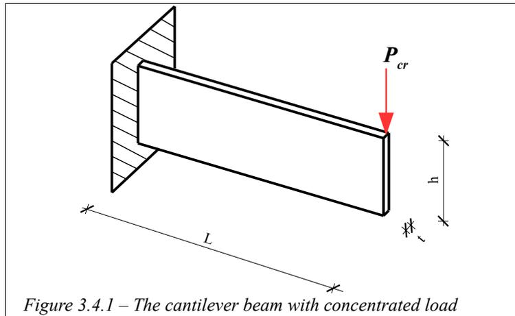
Figure 3.4.1 – The cantilever beam with concentrated load
