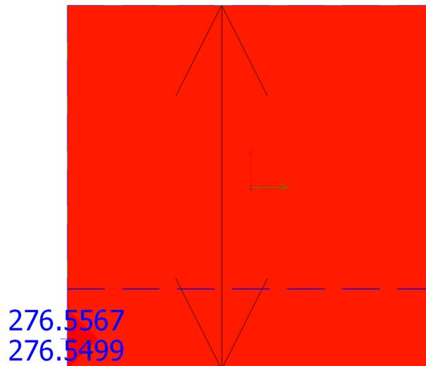
Figure 9.2.2.21 – The  $a_{s\xi}$  required reinforcement at the bottom for hyperbolic bending with non-orthogonal reinforcement [mm<sup>2</sup>/m]
