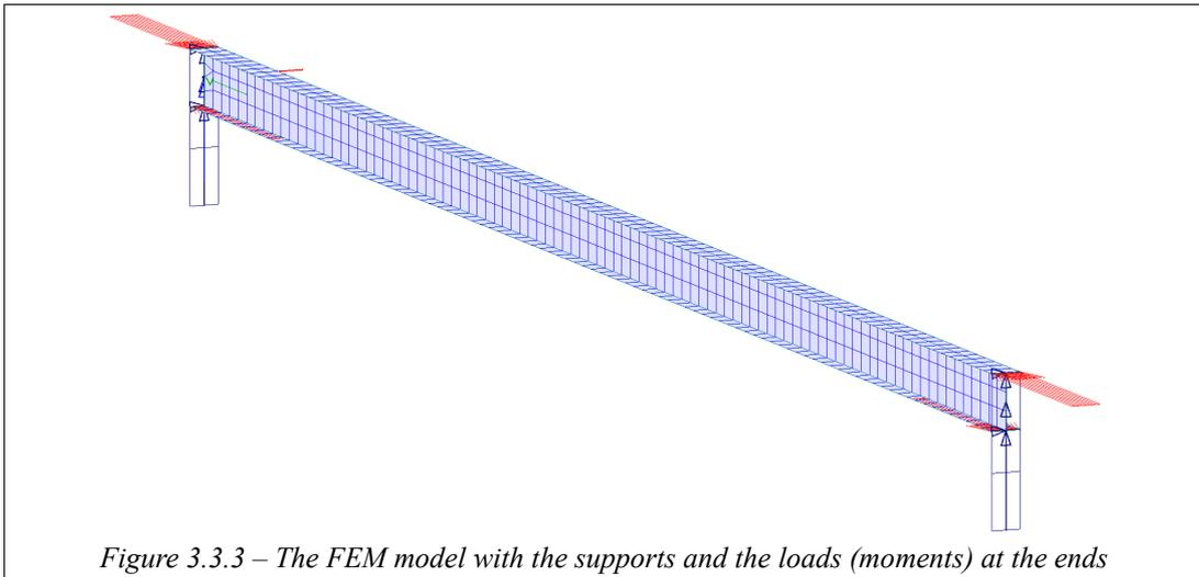
From the FEM-Design stability calculation the critical moment value for this lateral torsional buckling problem is:
