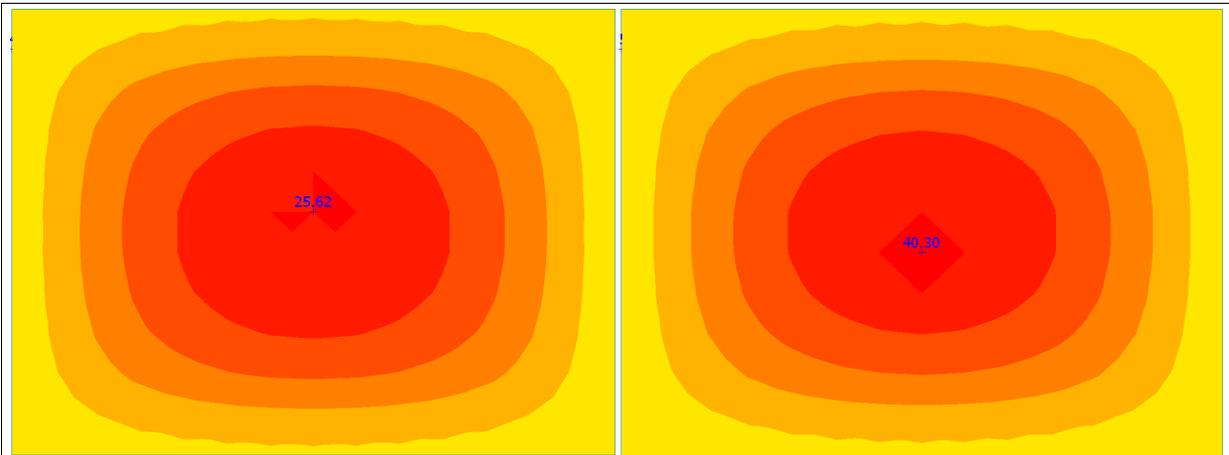
Figure 2.2.4 – The  $m_y$  [kNm/m] moment with 1<sup>st</sup> and 2<sup>nd</sup> order analysis
