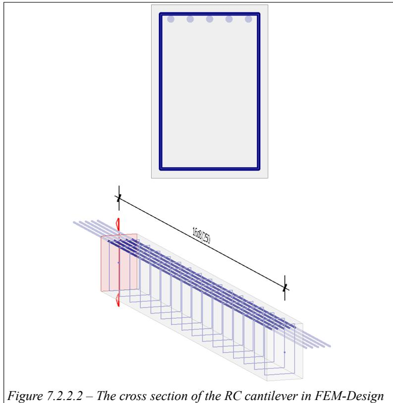
Figure 7.2.2.2 – The cross section of the RC cantilever in FEM-Design
