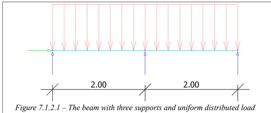
In first part of this case the maximum deflection comes from the following formula considering only the bending deformations in the beam:
