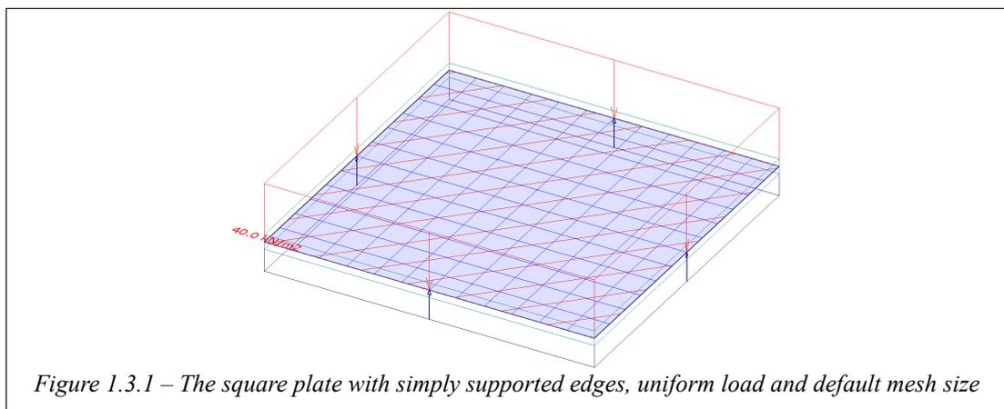
Figure 1.3.1 – The square plate with simply supported edges, uniform load and default mesh size
