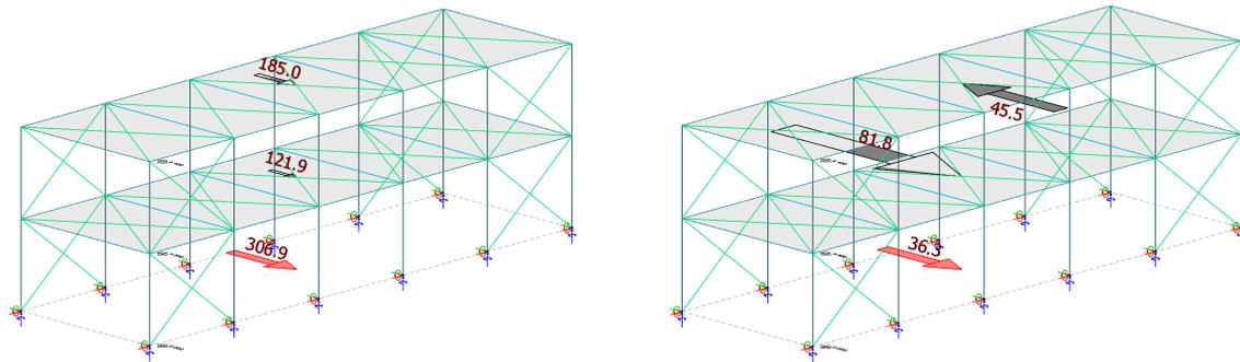
Figure 5.3.7 – The equivalent forces respect to the storeys and the base shear forces for the first two mode shapes [kN]
