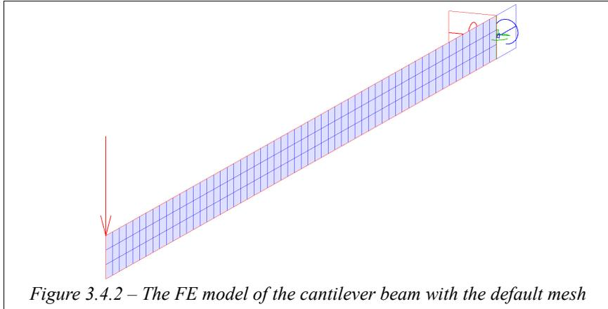
Figure 3.4.2 – The FE model of the cantilever beam with the default mesh
