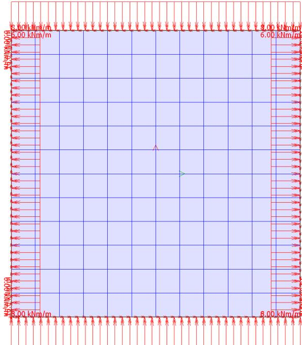
Figure 9.2.2.12 – The slab with the edge loads for pure stress state
