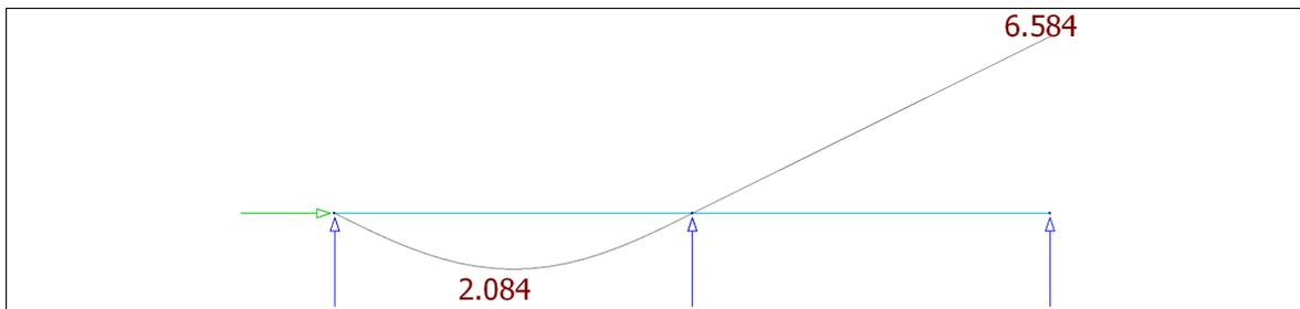
Figure 7.1.2.12 – The deflection of the beam when the right support only bear compression (partial load)
