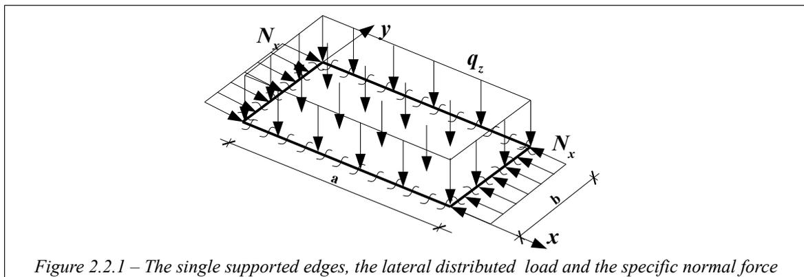
Figure 2.2.1 – The single supported edges, the lateral distributed load and the specific normal force
