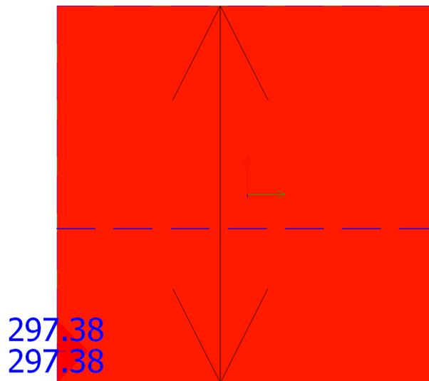
Figure 9.2.2.6 – The  $a_{s\xi}$  required reinforcement at the bottom for elliptic bending with orthogonal reinforcement [mm<sup>2</sup>/m]
