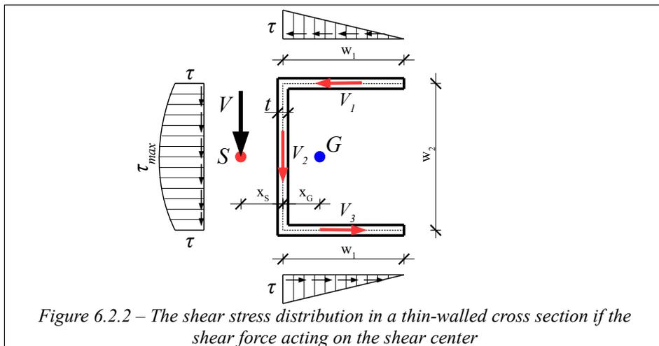
Figure 6.2.2 – The shear stress distribution in a thin-walled cross section if the shear force acting on the shear center
