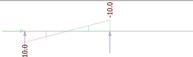
Figure 7.1.2.13 – The shear diagram of the beam when the right support only bear compression (partial load)
