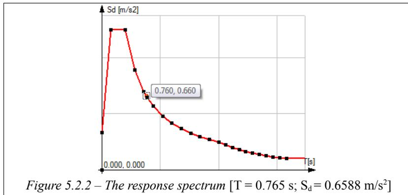
Figure 5.2.2 – The response spectrum [T = 0.765 s; S<sub>d</sub> = 0.6588 m/s<sup>2</sup>]
