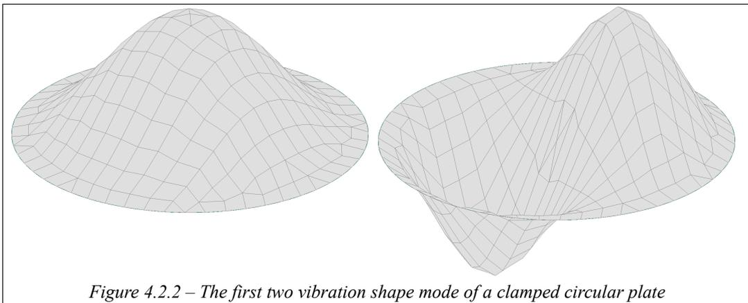
Figure 4.2.2 – The first two vibration shape mode of a clamped circular plate
