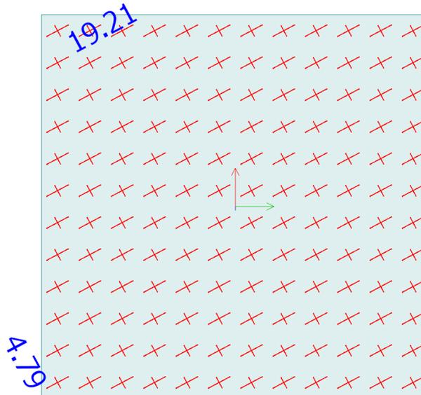
Figure 9.2.2.3 – The  $m_1$  and  $m_2$  principal moments and their directions in the slab [kNm]
