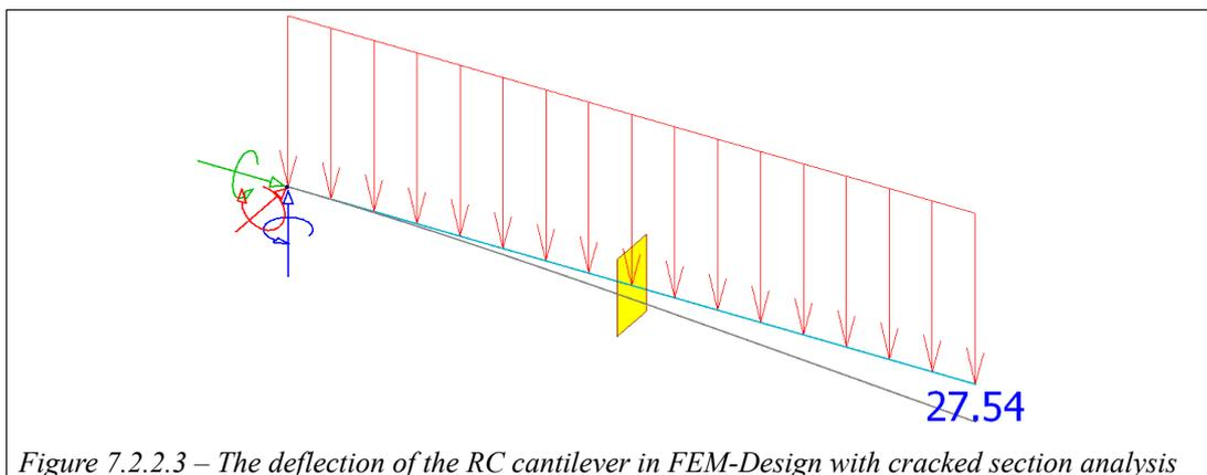
Figure 7.2.2.3 – The deflection of the RC cantilever in FEM-Design with cracked section analysis
