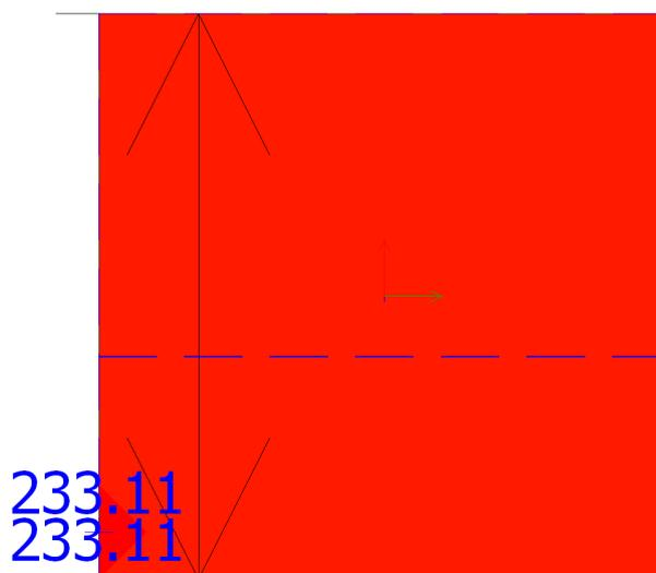
Figure 9.2.2.10 – The  $a_{s\xi}$  required reinforcement at the bottom for elliptic bending with non-orthogonal reinforcement [mm<sup>2</sup>/m]
