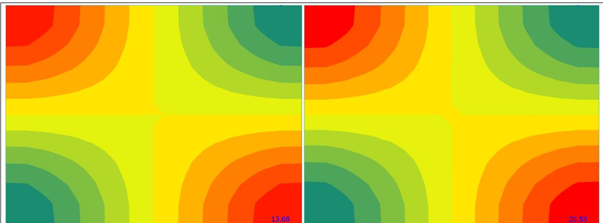
Figure 2.2.5 – The  $m_{xy}$  [kNm/m] moment with 1<sup>st</sup> and 2<sup>nd</sup> order analysis
