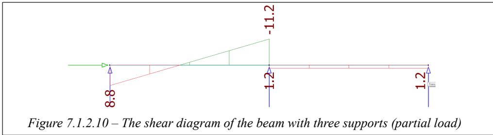
Figure 7.1.2.10 – The shear diagram of the beam with three supports (partial load)
