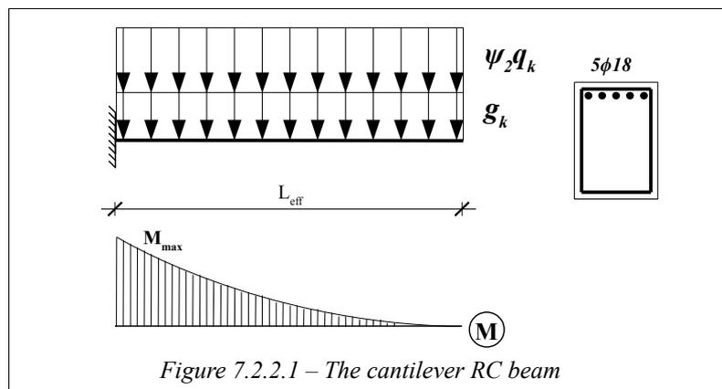
Figure 7.2.2.1 – The cantilever RC beam
