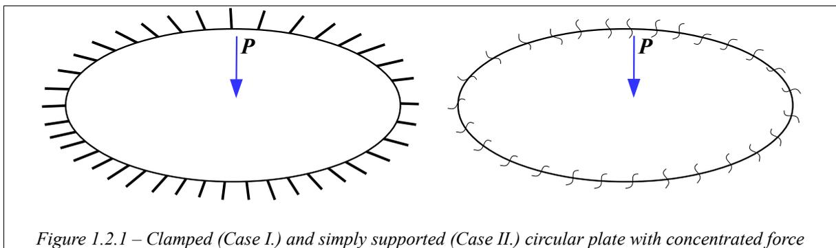
Figure 1.2.1 – Clamped (Case I.) and simply supported (Case II.) circular plate with concentrated force
