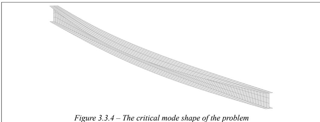
The difference between the two calculated critical moments is less than 1%.
