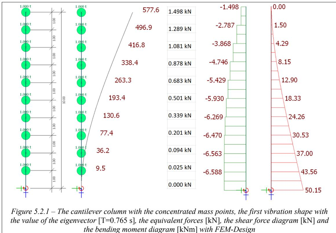
Figure 5.2.1 – The cantilever column with the concentrated mass points, the first vibration shape with the value of the eigenvector [T=0.765 s], the equivalent forces [kN], the shear force diagram [kN] and the bending moment diagram [kNm] with FEM-Design
