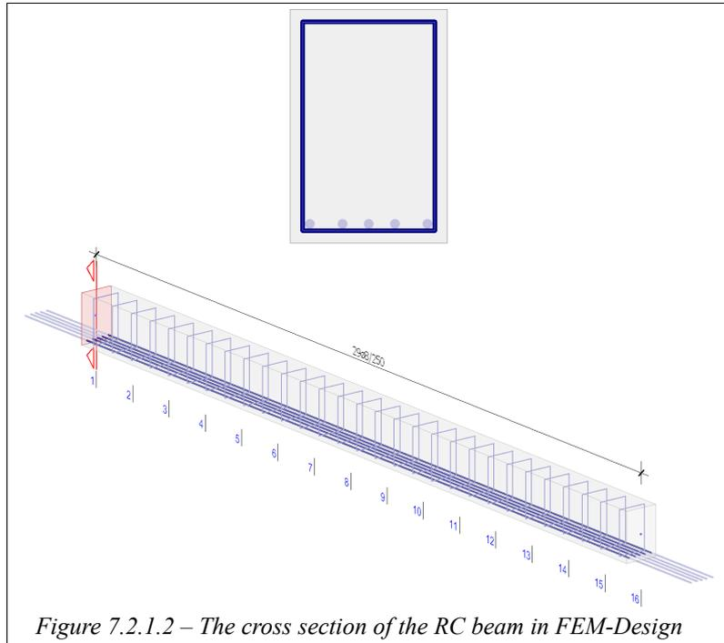
Fig. 7.2.1.2 shows the applied cross section and reinforcement with the defined input parameters.
