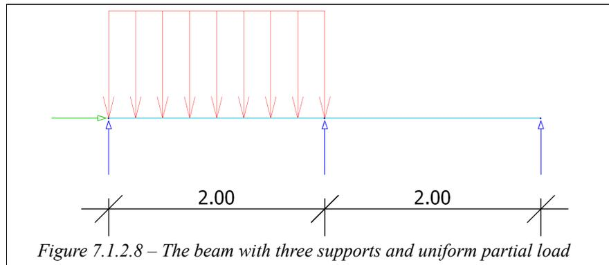
The extremums of the deflection come from the following formulas considering only the bending deformations in the beam (without signs):
