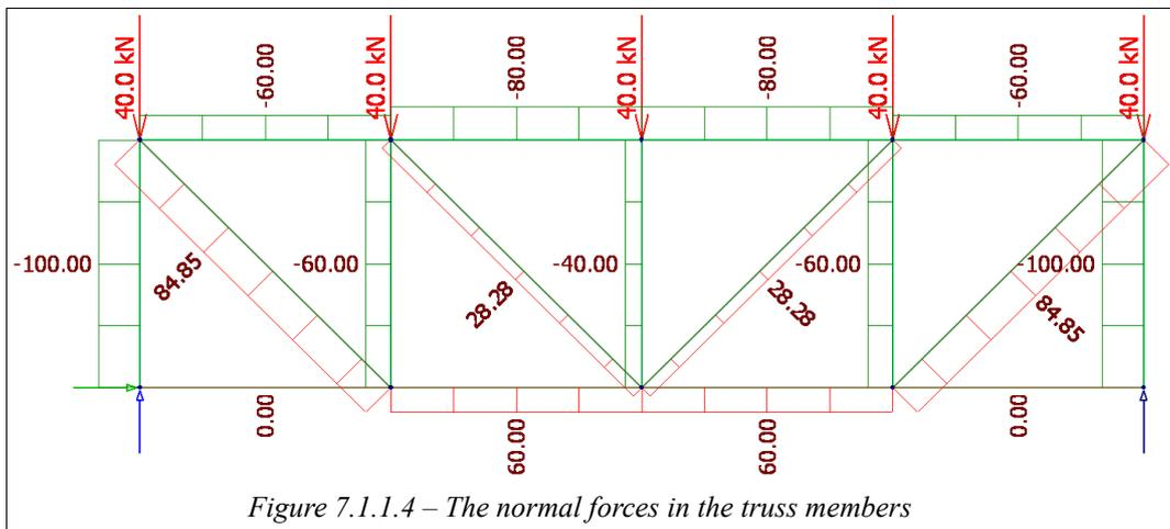
Figure 7.1.1.4 – The normal forces in the truss members
