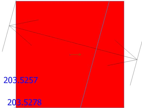
Figure 9.2.2.22 – The  $a_{s\eta}$  required reinforcement at the top for hyperbolic bending with non-orthogonal reinforcement [mm<sup>2</sup>/m]
