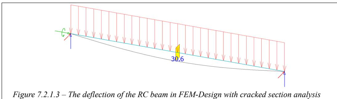
Fig. 7.2.1.3 shows the deflection after the cracked section analysis. The deflection of the beam model in FEM-Design:
