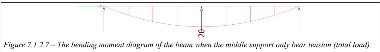
The differences between the calculated results by hand and by FEM-Design are less than 2%.
