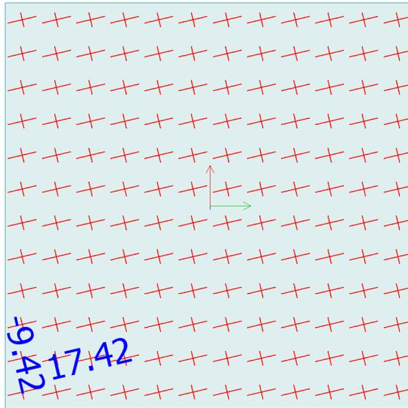
Figure 9.2.2.14 – The  $m_1$  and  $m_2$  principal moments and their directions in the slab [kNm]
