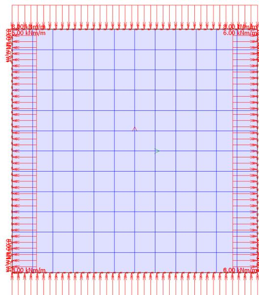
Figure 9.2.2.1 – The slab with the edge loads for pure stress state
