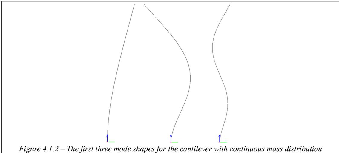
The differences between the analytical and FE solutions are less than 2 %.
