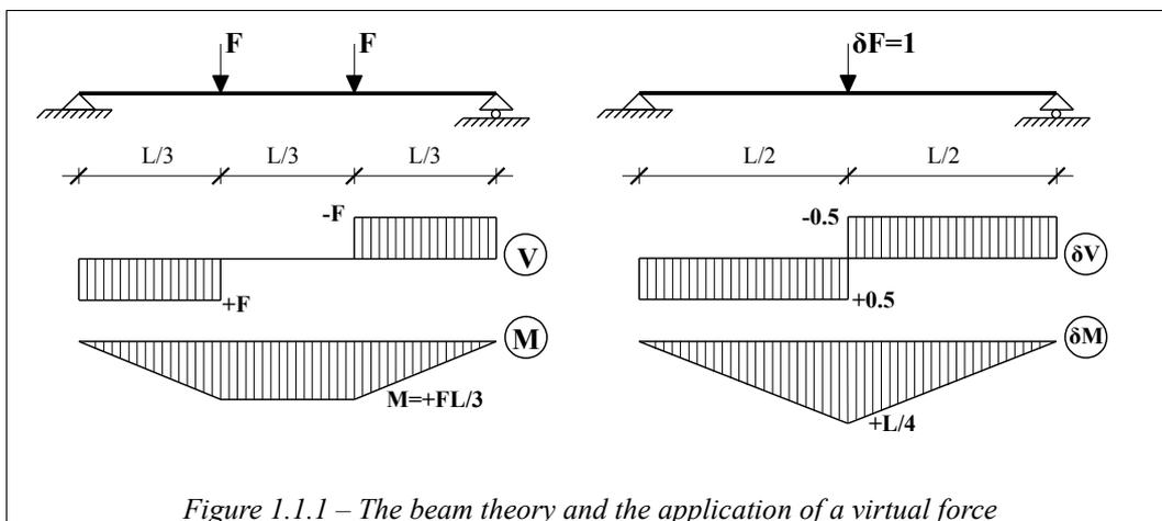
Figure 1.1.1 – The beam theory and the application of a virtual force
