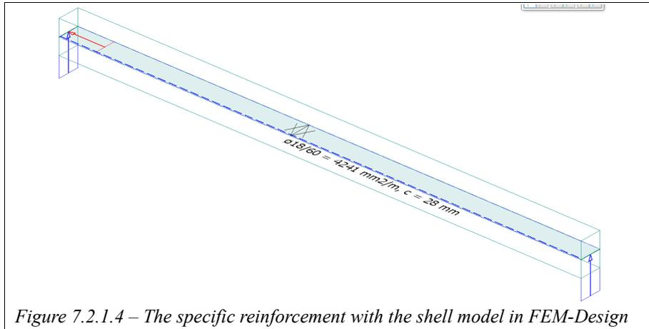
Figure 7.2.1.4 – The specific reinforcement with the shell model in FEM-Design
