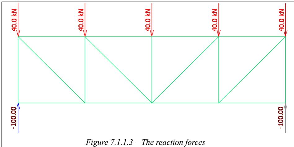
Figure 7.1.1.3 – The reaction forces
