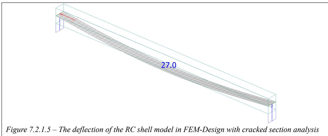
Figure 7.2.1.5 – The deflection of the RC shell model in FEM-Design with cracked section analysis
