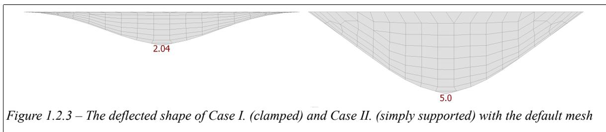
Fig. 1.2.3 shows the two deflected shape in side view. The different boundary conditions are obvious based on the two different displacement shape. The differences between the analytical solutions and finite element solutions are less than 5% but the results could be more accurate if the applied mesh is more dense than the default size.
