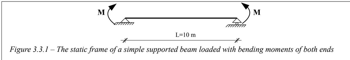
Figure 3.3.1 – The static frame of a simple supported beam loaded with bending moments of both ends
