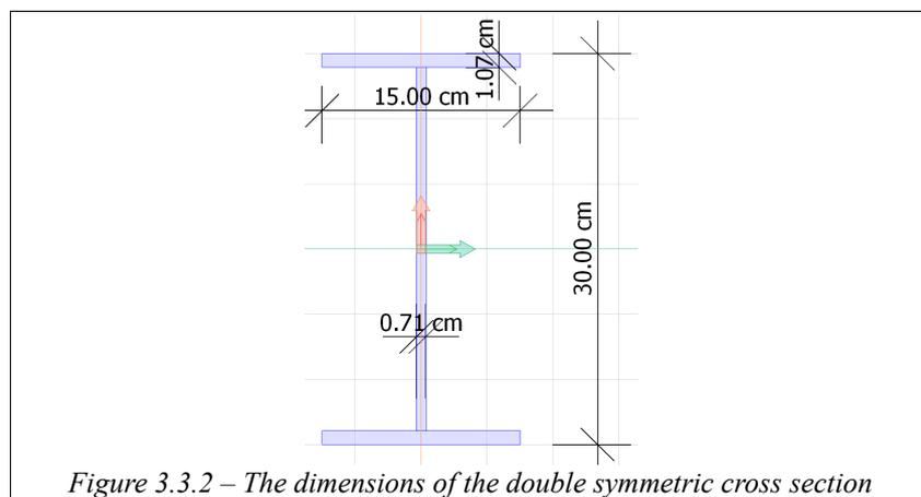
Figure 3.3.2 – The dimensions of the double symmetric cross section
