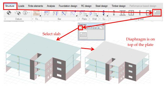
To consider the diaphragmas in the calculation the User needs to check "Apply diaphragms in analysis" option under *Calculate* dialog.
