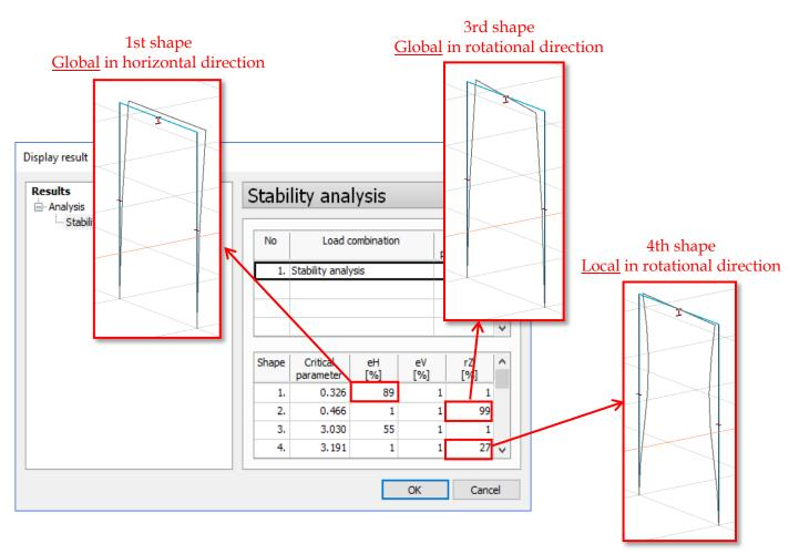
Displaying the result (see the leftmost inset above) and examining the buckling shape shows that this is indeed a case of global buckling with the horizontal displacement of the frame's top.
