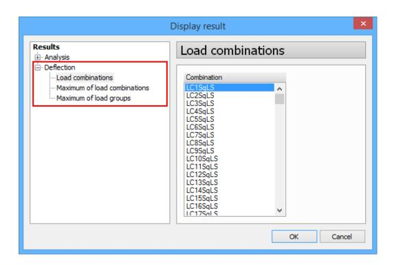
Due to the fact that the limit values of the calculation are controlled by the Deflection lengths, the result is constant along them. In other words we have one (dominant) utilization value for each Deflection length. Results for *Maximum of load combinations* and *Maximum of load groups* are only displayed on the undeformed shape of the structure.
