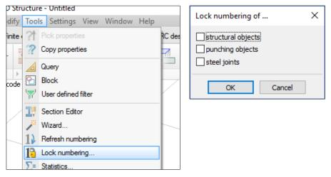
When the numbering of a selected object type is locked, the position number of individual elements will remain the same. The maximum position number is saved for all IDs, so position numbers less than that will not be used in the future, even if some items are deleted.
