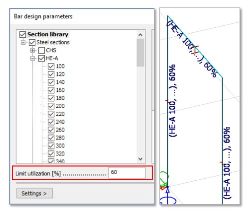
Status of bars with utilization less than 100% but more than the specified limit value will be displayed by a yellow tick in the *Utilization* dialog
