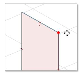
Snapping to surface is not enabled in *Wireframe* view mode. The point will instead snap to the User Co-ordinate System.
