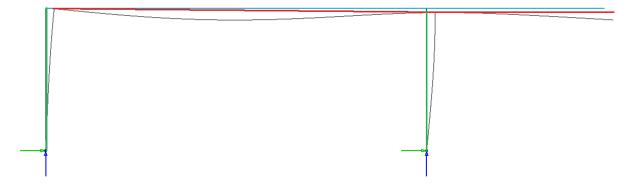
In the midspan we should use the Simply supported option, where we eliminate the rigid body motions in such a way that we connect the endpoints of the length, and measure the deflections of the middle sections from this imaginary line (red skew line on the picture above).
