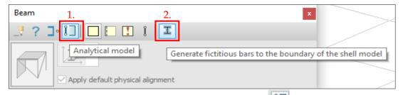
When creating a beam or column, (1.) select *Shell model* (1.), then (2) turn the option on or off as desired.
